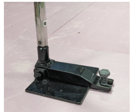
Figure 1 – The proper way to place the pull tester around a tie to be tested
